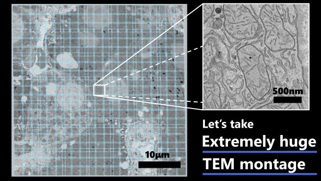
LLP makes it possible to take high quality TEM montage image (which is an image of large sight constructed of multiple images of small sight) of widespread area by a combination use of deflector and motor driving.
