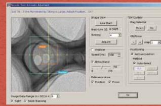
Assist functions for the sequential tilted image acquiring Algorithms corresponding to inherent problems, such as correction of shifted positions when specimens are tilted, and maintenance of the focus are provided. Furthermore, fine adjustment with manual operation is also available. Therefore, it is possible to acquire your favorites sequentially.
