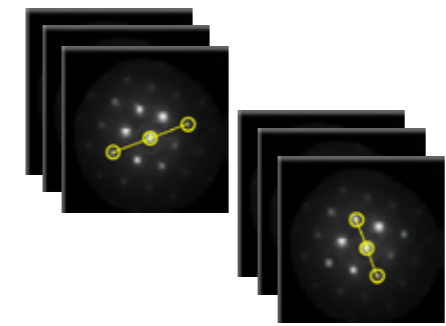
Pick a reference point and then measure the changes in the distance between correlated diffraction spots on each of recorded diffraction patterns.
