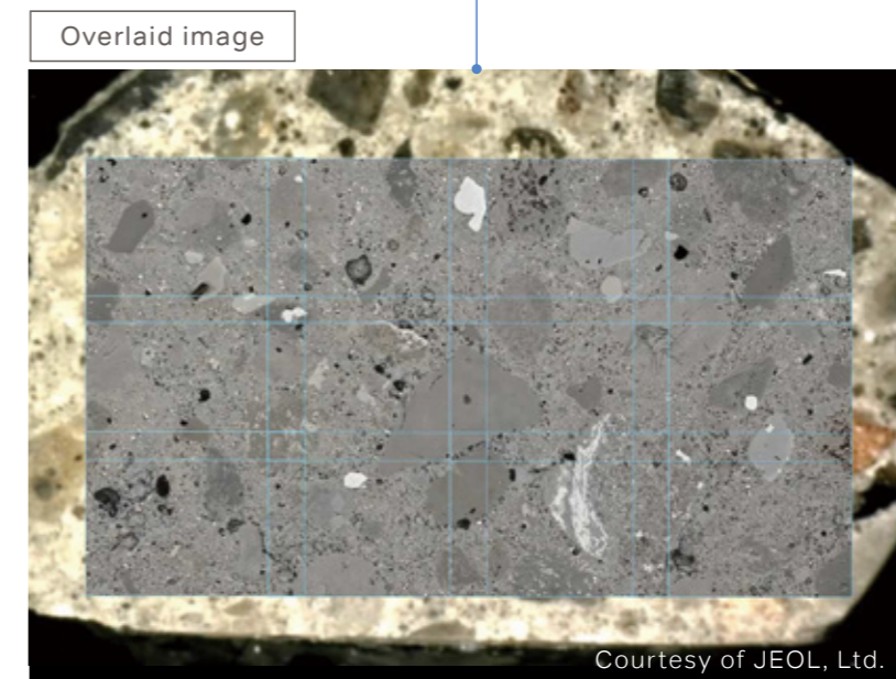
Simple operation creates an informative overlaid image from a montaged SEM image and an optical microscopy image.
