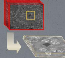
In Array Tomography, the observation target can slightly rotate. StackerNEO corrects this rotation and aligns based on a feature matching algorithm.
