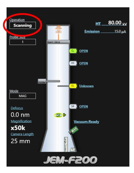
Make sure that TEM Center is running, and the operation mode is STEM mode (scanning mode) but not TEM mode.
