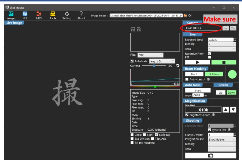
Make sure Shot Meister G2 is communicating with the correct camera, especially in a multi-camera environment. If Shot Meister G2 is communicating with wrong camera, stop using immediately and contact us via contact form of TEMography.com.
