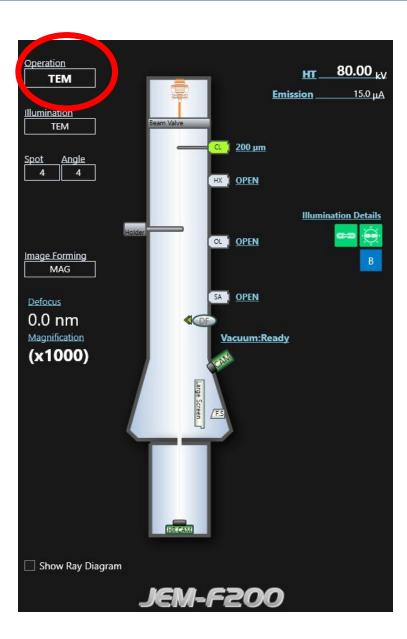
Make sure that TEM Center is running, and the operation mode is TEM mode but not STEM(Scanning) mode.
